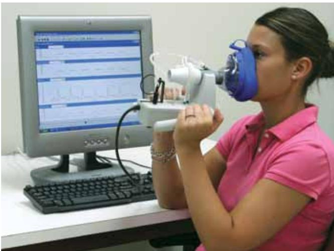
*Aerodynamic and intraoral pressure measurements are used in combination with acoustic and stroboscopic assessment in leading voice labs.*
