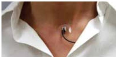
*APM data is captured by means of a throat sensor (accelerometer) attached to the neck and connected to the hardware module that is worn by the client.*
